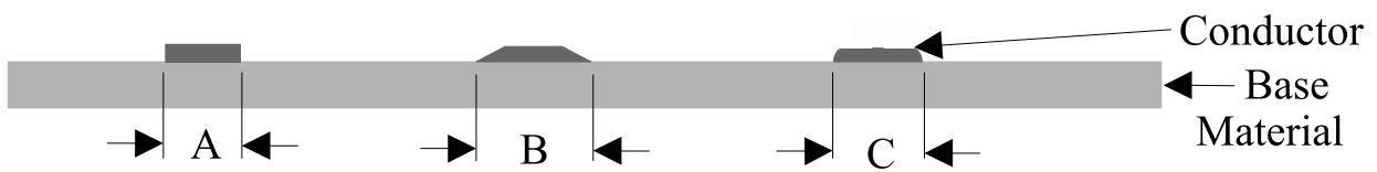
Figure 12.1 Measuring Conductor Trace Average Width (Side-View)
