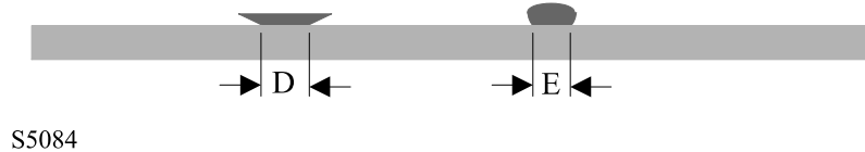
Figure 24.3 Measuring Conductor Trace Average Width (Cross Section-View)
