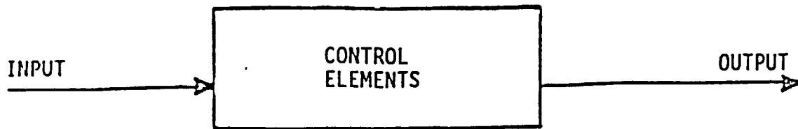
FIGURE 9 - Open Loop Control System
