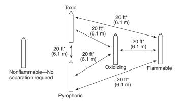
$<sup>^*</sup>$  The 20-ft (6.1-m) distance may be reduced without limit when separated by a barrier of noncombustible materials at least 5 ft (1.5 m) high that has a fire resistant rating of at least  $\frac{1}{2}$  hour.
