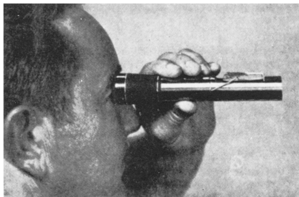
FIGURE A.6.2.2(b) Holding this Type of Refractometer Up to a Light Source to Take a Reading Where the Dark Field Intersects the Numbered Scale.
