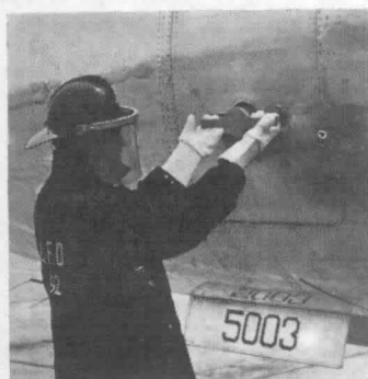
Figure A-25C. Normal entry at main entry door — first pull door handle outward.
