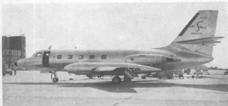
Figure A-25B. The JetStar is typical of modern turbine powered jet transports carrying a two-man crew and up to eight passengers.
