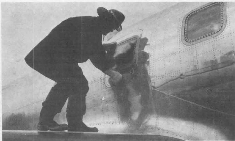
Figure A-25F. The fourth window from the front on each side of the JetStar fuselage is an emergency hatch. To open from the outside, push in on the bottom of the flush latch plate underneath the bottom edge of the window. Push inward.
