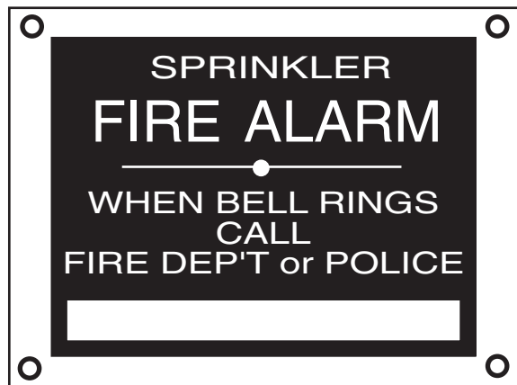
FIGURE A.8.17.1 Identification Sign.
