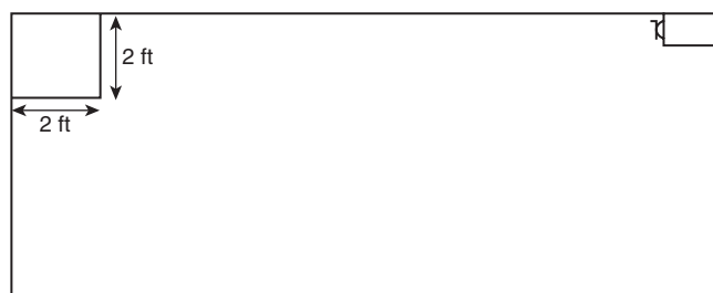
FIGURE A.8.10.7.1.6 Permitted Obstruction on Wall Opposite Residential Sidewall Sprinkler.
