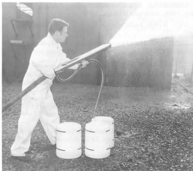
Figure A-1-4(a) Air foam hose nozzle with built-in eductor.
