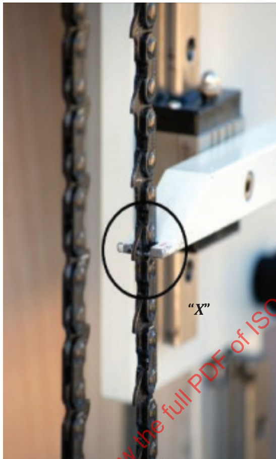
b) Detailed view of the chain mounting (Detail “X” of Figure 2 )
