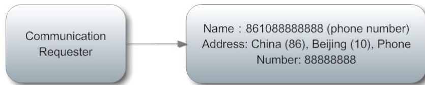
Figure 1 — Addressing Mode NAS (Telecom network)
