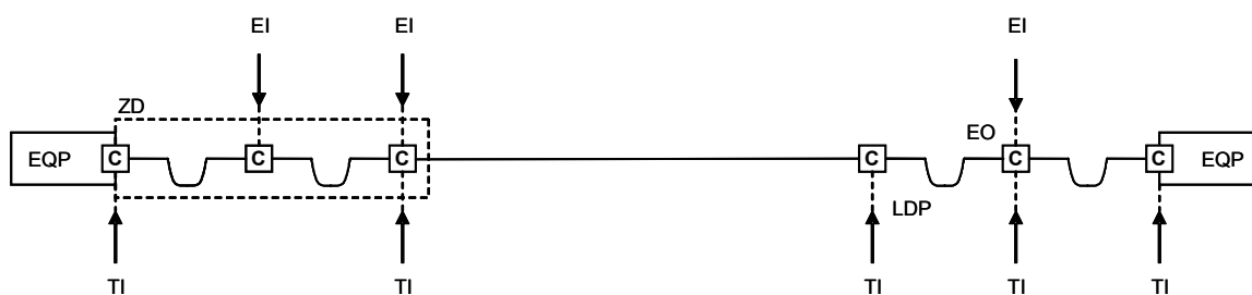
Figure 5a – Zone distribution cabling
