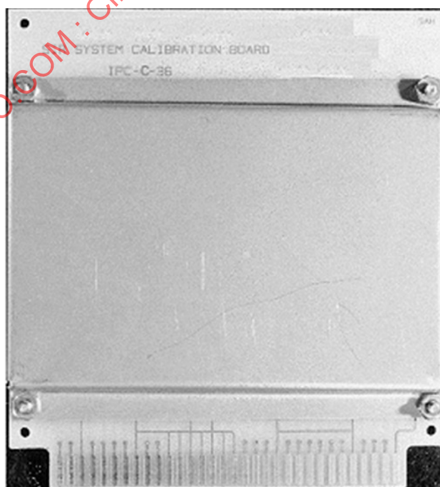
Figure 3 — Resistor verification board with protective cover
