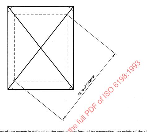
NOTE — Measurement area of the screen is defined as the central area formed by connecting the points of the diagonals that are located from the corners at a distance of 10 % of the screen diagonal lengths. That is, the area within the dashed rectangle. If the corners of the screen are rounded, the length of the diagonals and the points from which readings are taken shall be calculated from the extrapolated edges of the screen. Screens may be either square or a vertical or horizontal rectangle.
