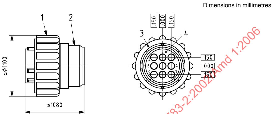
The optional in-cab connector plug specifications are met by AMP 206708<sup>1 2)</sup>.
