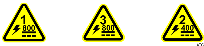
Figure G.9 – Examples of DC zones labels
