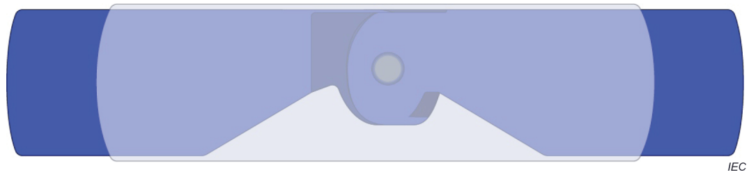
Figure E.3 – Specimen holder covered with silicone
