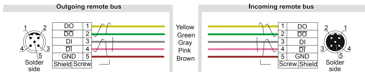
Figure A.5 – M12 circular connector pin assignments
