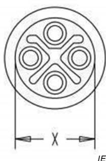
Figure A.1 – Diameter of the female connector body
