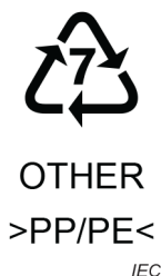
Figure 2 – Marking of polypropylene-polyethylene copolymer battery components
