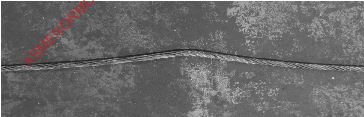
Figure 30-1.8.2-3 Distortion of Rope Structure — Dogleg
