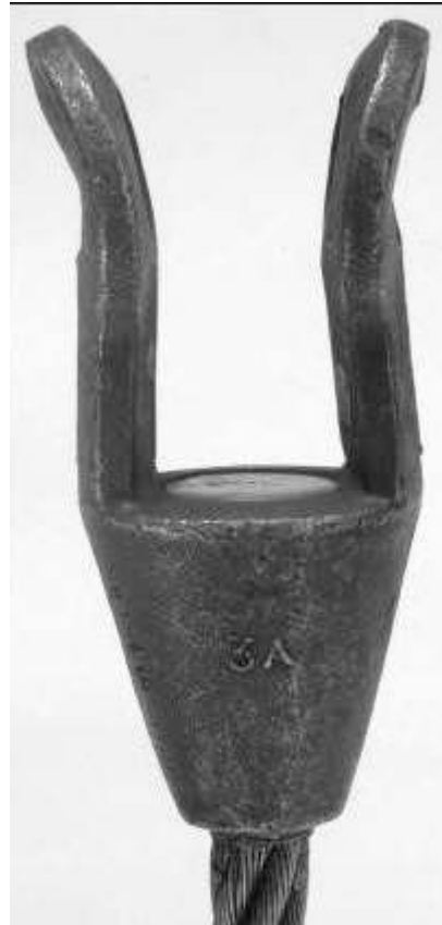
Figure 30-1.8.2-9 Damaged End Terminations
